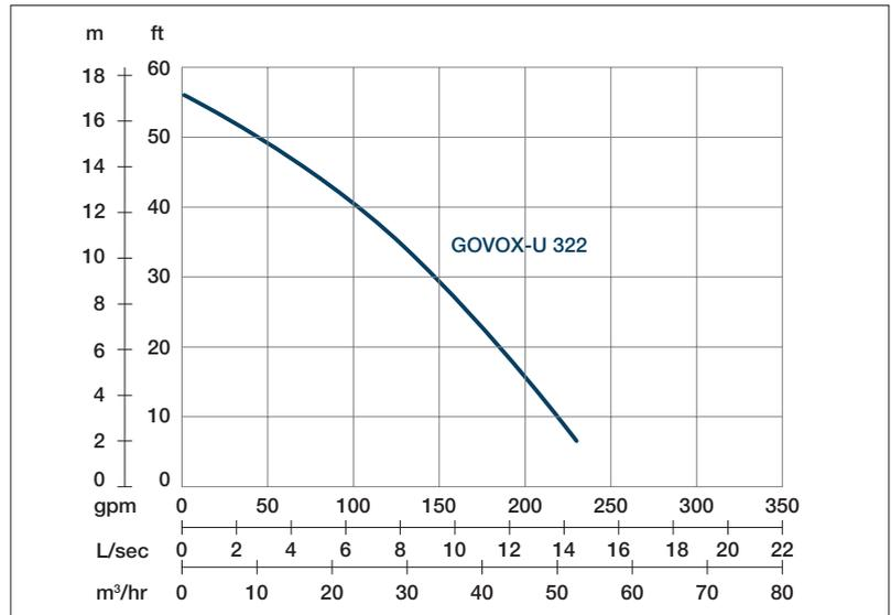
Shaft Speed : 2850 rpm
